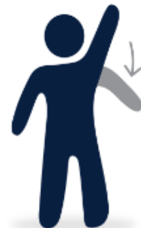
Is it safe to cross the track? Arm Vertical–Wait not safe Arm dropped–Cross now
