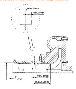
**DRAWING 2: TURBOCHARGER RESTRICTOR ALTERNATE MOUNTING**
